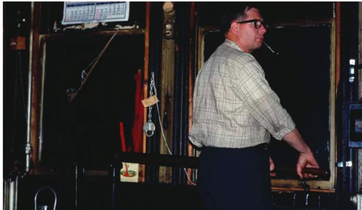
While the interlocking plant at Athens Tower was electrically operated, the crossing gates for Main Street were not. A towerman works the pump lever that raised and lowered each set of gates individually. He had three minutes to lower three sets of gates. Robert Archer
