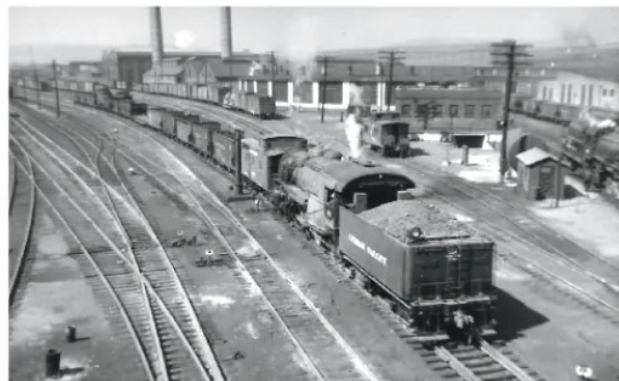
Sayre Yard was also a major shop complex for the Lehigh Valley. It boasted a huge roundhouse and facilities for maintenance and heavy repairs of the railroad's steam locomotive and rolling stock fleets. Here, the yard switcher assembles a train. David Marcham
