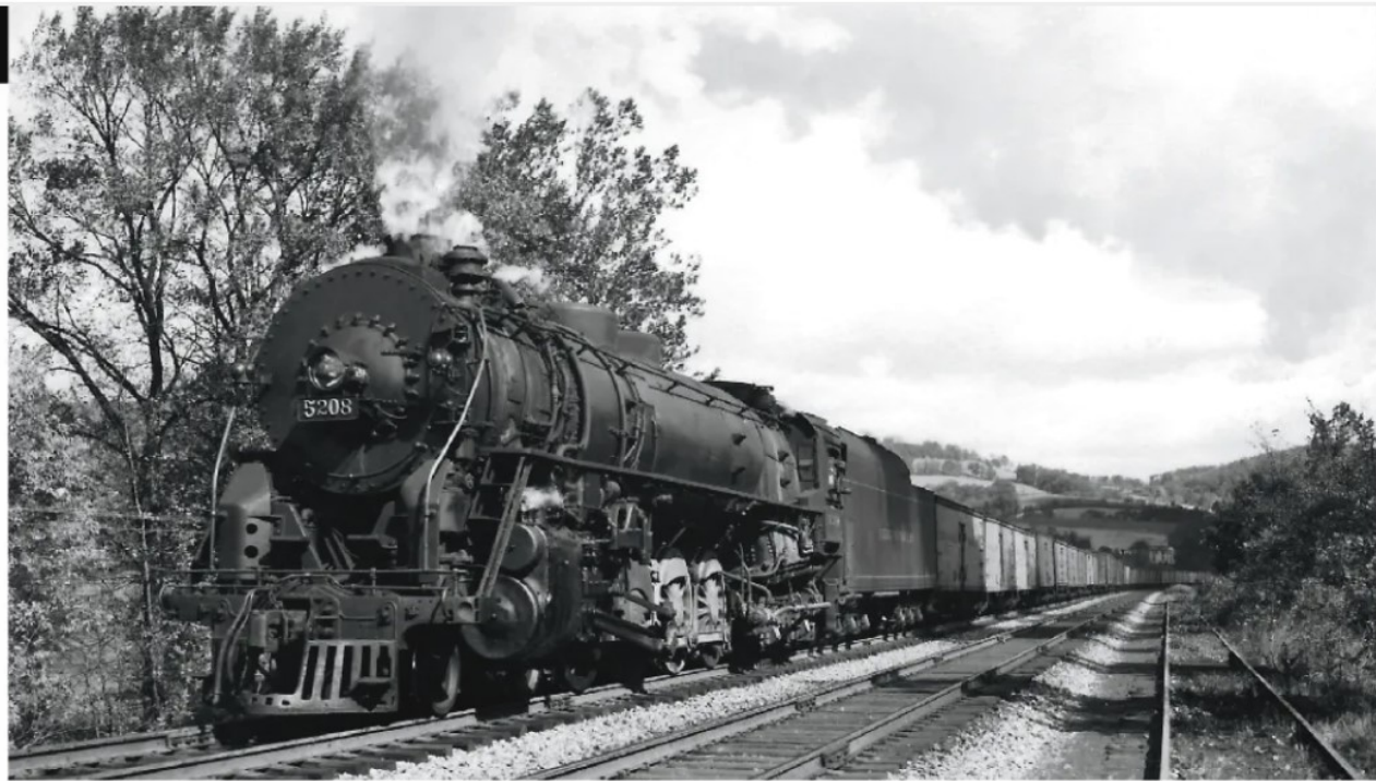
One of Lehigh Valley's T-2 4-8-4s is in charge of a symbol freight of reefers near Rummerfield, Pa., east of Towanda. It took some burly power to keep trains on time given the topography of the line that followed the curvy Susquehanna River. Donald Furler
