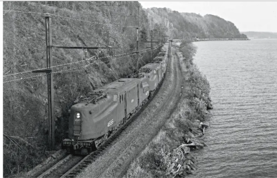
Four Conrail GG1s take mixed freight WIEN (Edge Moor Yard, Wilmington, Del.-Enola, Pa.) west at Safe Harbor, Pa., on Nov. 4, 1979. The electrics were long in the tooth, so Conrail often dispatched freights with four motors, in the hope that at least one would be running at the end of the trip.
